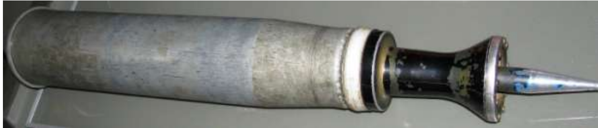
Figure 2: A 105mm APFSDS round. The sabot is the black cone surrounding the rod which itself extends back to the ogive in the cartridge.
