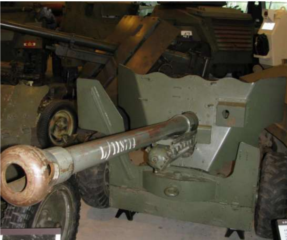
Figure 5: The museum's British 6-pounder AT gun. Its 90-degree traverse and 1000 lb weight made it easily manageable by its crew. Even when it was outclassed by German armour late in the war it still provided good service as an infantry support weapon.
