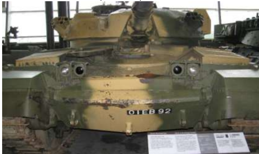
Figure 20: Massive frontal armour - the museum's Chieftain tank. Smoke grenade launchers for defense against missile attack are attached to the turret.
