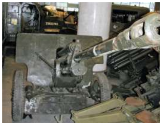
Figure 7: The ZiS-3. The improvised 75mm field gun was married to a light 57mm AT gun carriage necessitating the use of a muzzle brake. This resulted in a low-profile light gun that worked well in the AT role.
