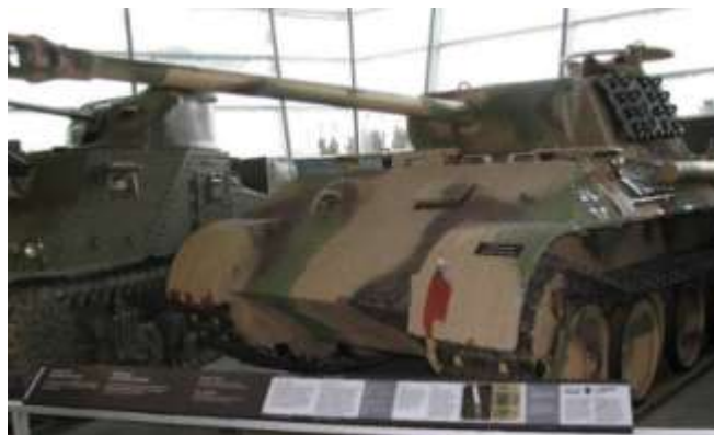
Figure 3: The KwK 42/L70 mounted in the Museum's Mk V "Panther" tank. The large turret permitted 360 degree firing at a cost of a large chassis and weight.
