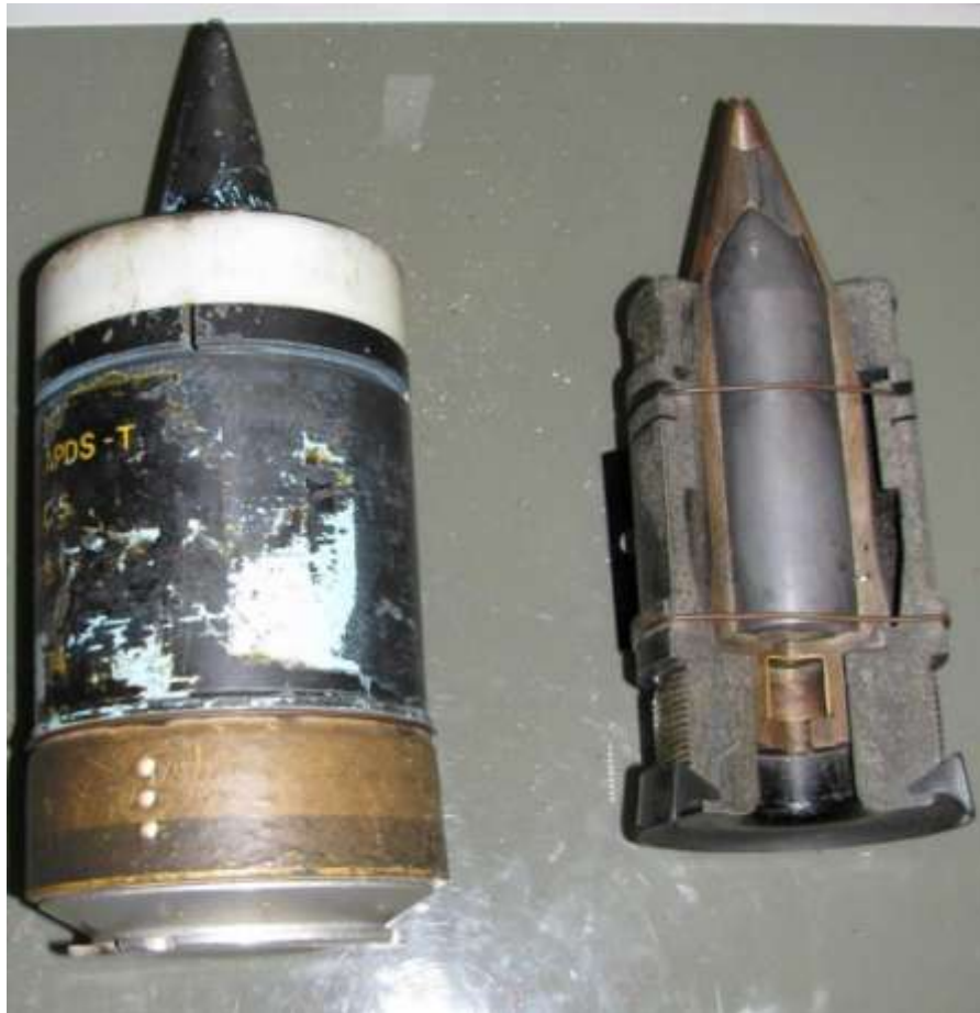
Figure 1: An armour piercing shot with a disposable sabot cut away to show its construction. The rigid shot has an armour piercing cap and then is encased in a soft metal outer layer with a ballistic nose cap. A 105mm version is to the left of it with its Armor Piercing Disposable Sabot – Tracer marking clearly visible.
