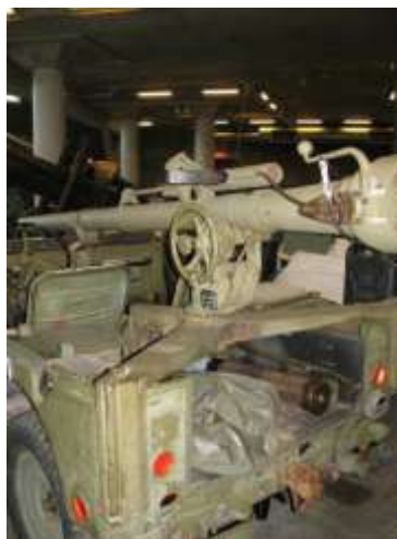
Figure 14: A US 106mm BAT mounted on a jeep. A recoilless rifle (with its perforated cartridge visible), its back-blast would be highly visible to its intended victim - making a first-round hit and a "shoot and scoot" capability highly desirable. The museum also has a similar Soviet designed weapon used by Syria.
