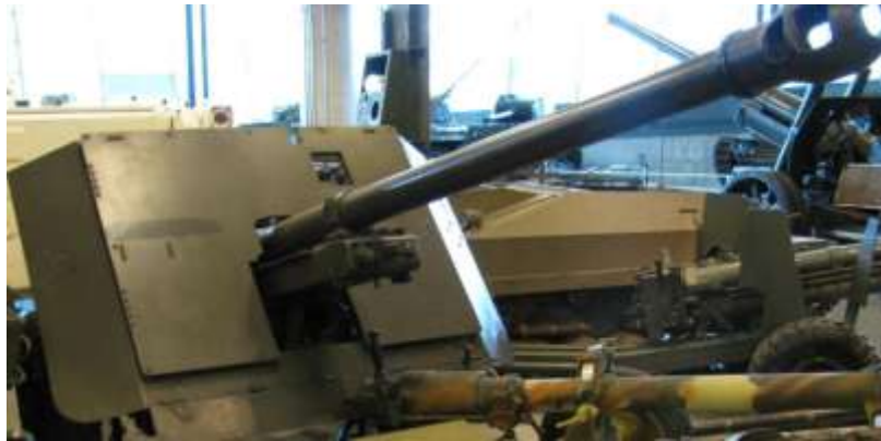
Figure 6: The 17-pounder AT gun. This had a similar and arguably better performance against armour than the German "88" but at 3 tons weight was not easily maneuvered on the battlefield.
