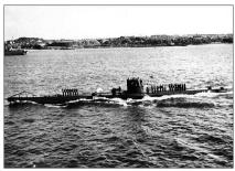
First launched in June 1936, the Type VII was the most successful of the war and formed the backbone of the U-boat force. Like many other military designs, the original Type VII was quickly modified to provide longer range, better performance and revised armament. These additional variants resulted in an improved torpedo attack boat (VII-C), minelayer (VII-D), supply boat (VII-F) and other variants such as Flak and repair boats.
